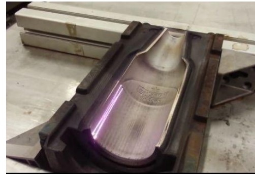
Mold oil removal
