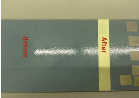
Plate paint removal
