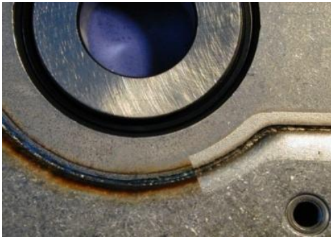
Welding line cleaning
