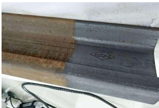
High-speed rail derusting
