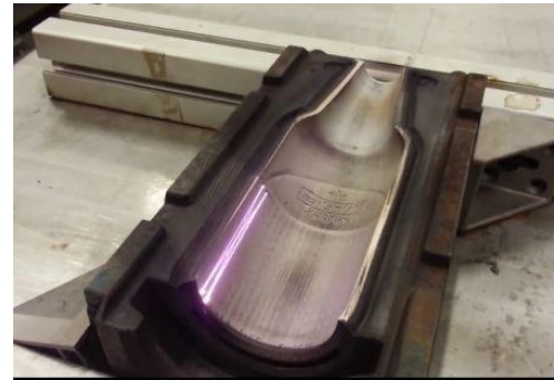
Mold oil removal
