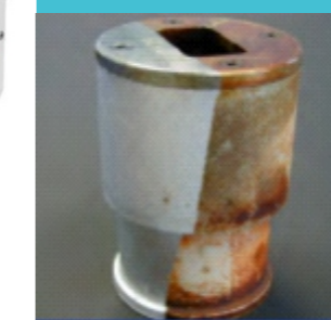
Rust removal from automobile parts
