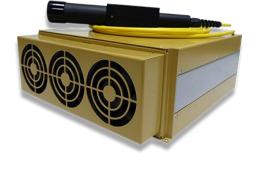
CINA Laser PYL/N nanosecond ytterbium fiber lasers provide average output power up to 500 W and adjustable pulse waveforms in the range of 2-500 ns. The lasers are triggered externally in a wide range of pulse repetition rates 1-4000 kHz, offers pulse energy of up to 2 mJ and the ability to scale average power independent of the energy.
